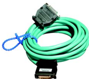
Connection cable Multiplexer – PLC TTY
